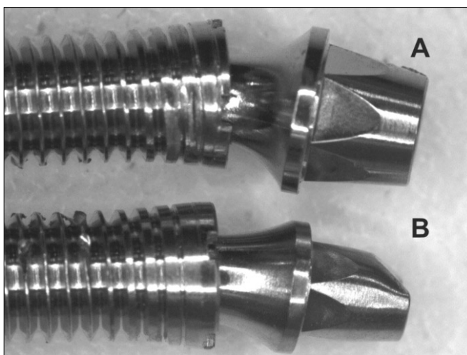
Fig. 3. Implant/abutment sets after mechanical test. A-4.8 mm abutment; B-3.8 mm abutment.
